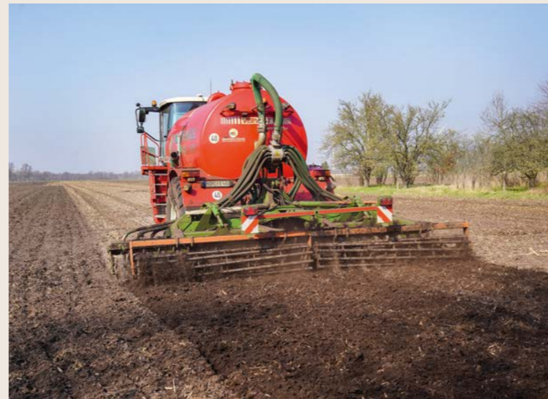
The Hydro-Trike injects the slurry directly into arable fields.
